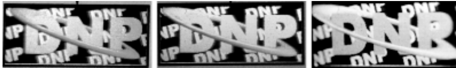
Figure 1. Reconstructed monochrome images of the CGH under white light. Pictures are taken from the: (a) left, (b) front, (c) right.
