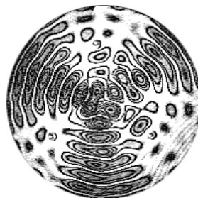
Figure 3. Bronze plate under dynamic load at 8.84Hz. A combination of real-time and time-averaged holography leads, with the addition of phase shifting, to excellent interference fringe visibility. The amplitude of adjacent vibration modes is in the range of 1.5µm.
