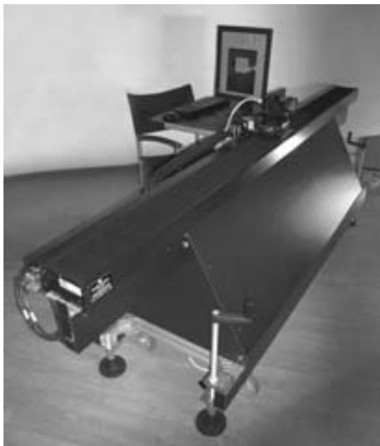
Figure 3. The VIP (video images with parallax) system.
