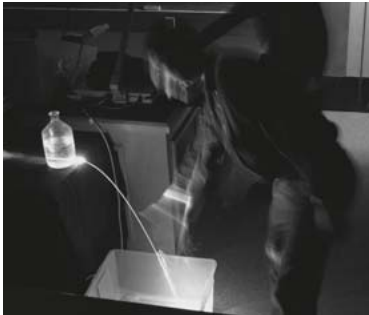
Figure 2. Dr. Bill Brocklesby demonstrates Tyndell's/Colladon's experiment, guiding light down a stream of water during the lecture.
