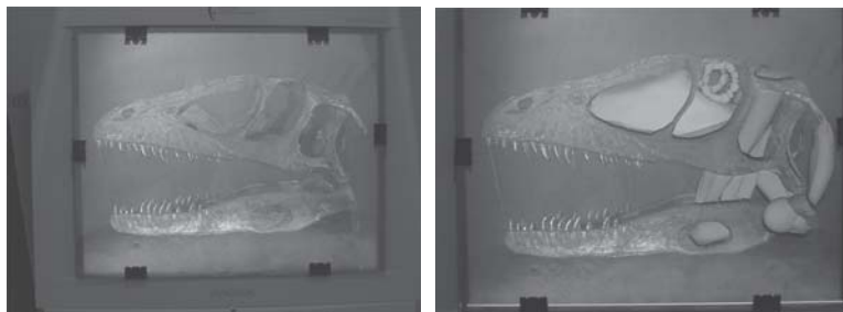
Figure 1. Rainbow hologram of a dinosaur skull combined with graphical representations of soft tissue and bones.
