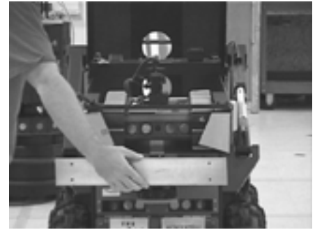
Figure 2. The mother uses daughter's camera (in the middle of the upper row of sonar disks) as a surrogate.
