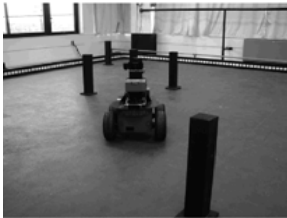
Figure 1. A snapshot from a lab-based SLAM experiment is shown on the left. This is displayed in schematic plan view on the right. The two robots sense features (indicated by crosses) in the lab environment and incorporate them into a global map. Each robot fuses the other's map by employing a fully decentralized form of the SLAM filter.
