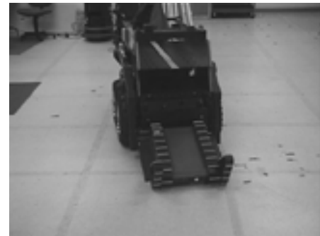
Figure 4. Next, she deploys the daughter, which then reverses into the bay so that her camera faces backward.
