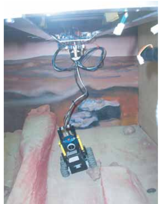
Figure 3. The hoist mechanism allows the tether to track the rover.
