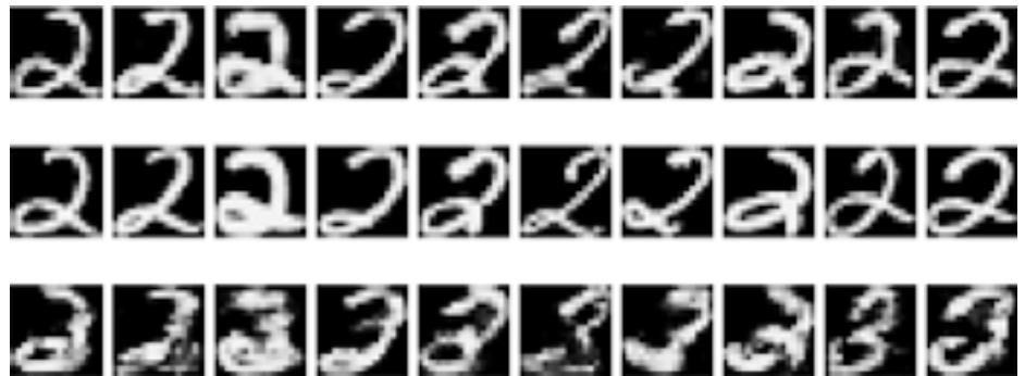
2. A demonstration of how important well-adapted feature detectors are to pattern recognition. The center row shows a set of 2s that were previously unseen by two networks, one trained on 2s, the other trained on 3s. The top row demonstrates how the network that "believes in 2s" can regenerate the numbers reasonably well (and so will be able to recognize them easily). The network trained on 3s, on the other hand, keeps trying to "fix" the 2s to look like the number it's expecting.
