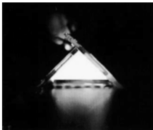
Figure 2. A mock up of the pyramid-shaped pixel structure was created by gluing polymer LEDs onto the inside of this prism (a scaled-up version of the design shape).
