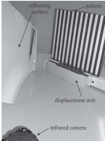
Figure 1. Setup for infrared deflectometry: infrared radiation is emitted as a pattern that is laterally shifted. The radiation is reflected from the part and observed by the infrared camera.
